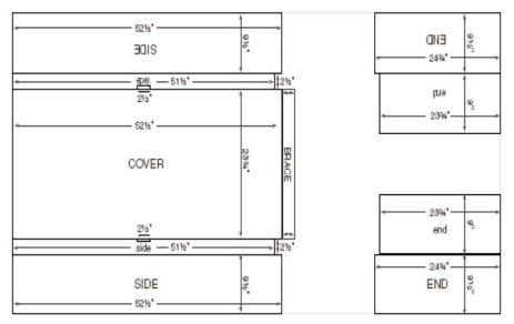
Dimensions shown are for a box 53½" outside (51½" inside), 24¾" outside (22¾" inside), and 9" of depth inside. Adjust dimensions to fit the specific stairs being installed.
