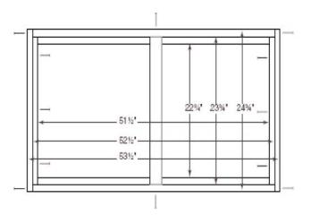
Assemble side pieces, end pieces, and brace as shown. The cover piece will drop in and be attached with adhesive and nails.
